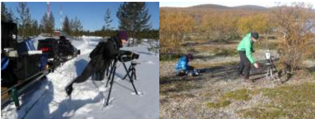
Figure 1.1. Field measurements with ASD (Analytical Spectral Device) HandHeld in winter in Sodankylä and in the autumn in Karigasniemi
