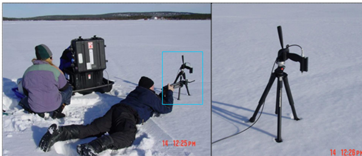
Image 1 Photograph showing the measurement set up for reflectivity measurements.
