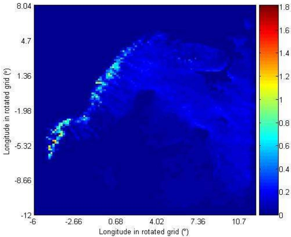
Figure 2. Snow depth in terms of water equivalent (m) within the domain on March 1<sup>st</sup> 2005.
